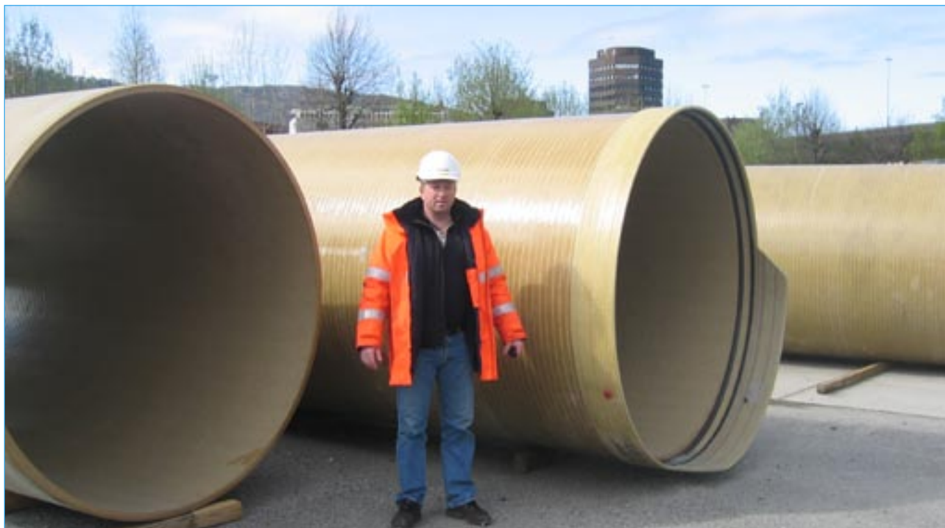
GUP rørene – 2 meter diameter
